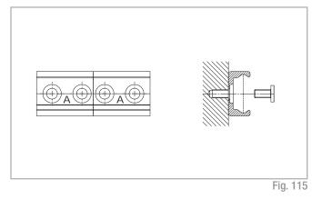
(3) Place the alignment fixture on the rail joint and tighten both set screws uniformly, until the raceways are aligned (see fig. 116).
