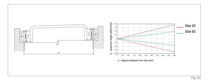
Even the K+U-system can be used in different arrangements. If the same example as with the T+U-system is observed (see pg. CR-41, fig. 60), this solution, in addition to the prevention of vibrations and moments, also enables the compensation of larger deviations in parallelism in the vertical direction, without negative consequences to the guide. This is particularly important for longer strokes as it is more difficult to obtain a correct vertical parallelism.
