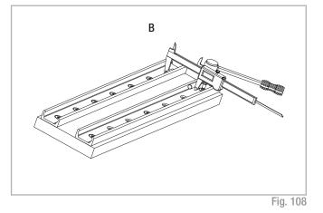
(4) Fasten the screw in Position C so that the distance of the raceways is as close to an average between the two values from A and B as possible.(5) Fasten all other screws and check the specified tightening torque of all fixing screws (see pg. CR-61, tab. 43).
