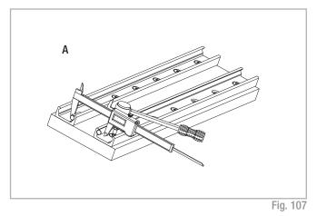
(3) Fasten the rail in Position B so that the distance between the raceways does not exceed the measured values in Position A while maintaining the tolerances (see pg. CR-63, tab. 45) for parallel rail installation.
