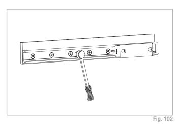
(2) Install a dial indicator so that the offset of the rail to a reference line can be measured. Now position the slider in the center of the rail and set the dial indicator to zero. Move the slider back and forth between each two hole spacings and carefully align the rail. Fasten the three center screws of this area now with the the specified tightening torque, see pg. fig. 103.(3) Now position the slider on one end of the rail and carefully align the rail to zero on the dial indicator.
