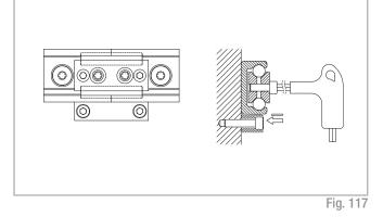
(6) Insert the key through the holes in the alignment fixture and tighten the screws on the rail ends.
