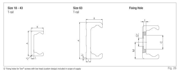
$\mathsf{Q}^1$  Fixing holes for  $\mathsf{Torx}^{\circledast}$  screws with low head (custom design) included in scope of supply
