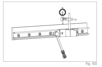
(4) Begin to tighten the screws as specified while moving the slider together with the dial indicator. Make sure that it does not show any significant deflection. Repeat this procedure from the other end of the rail.
