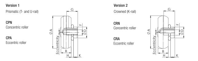
Seals: 2RS is the splash-proof seal, 2Z (2ZR for size 63) is the steel cover disc Note: The rollers are lubricated for life
