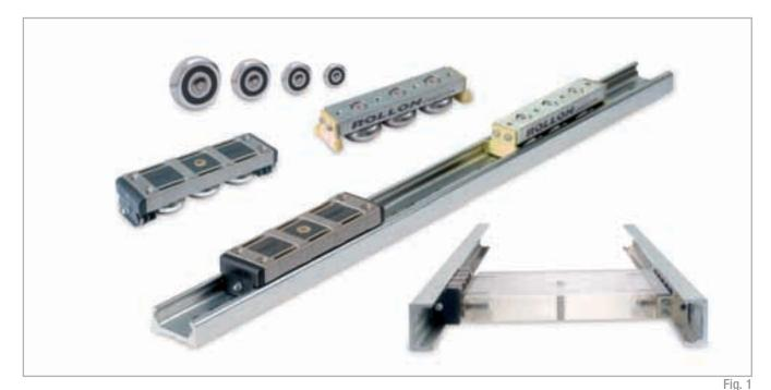
Compact Rail is the product family of guide rails consisting of roller sliders with radial bearings which slide on the internal, induction hardened and ground raceways of a C-profile made from cold-drawn roller bearing carbon steel.
