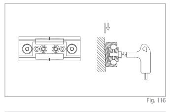
(5) The bottom of the rails should be supported in the area of the transition. Here a possible existing gap must be looked for, which must be closed if necessary for correct support of the rail ends by shims.
