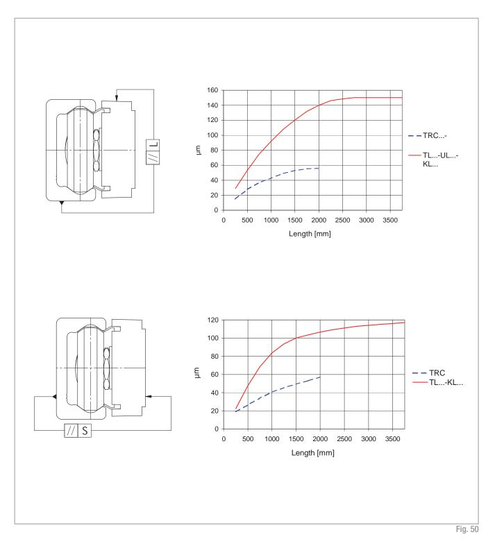
Deviation of accuracy with two 3 roller sliders in one rail
