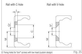
$\mathsf{Q}^1$  Fixing holes for  $\mathsf{Torx}^{\circledast}$  screws with low head (custom design) included in scope of supply V<sup>1</sup> Fixing holes for countersunk head screws according to DIN 7991
