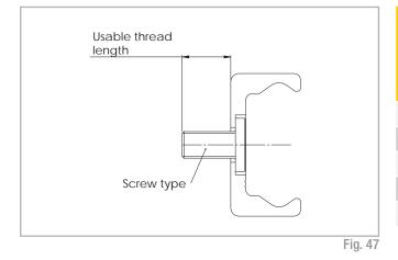
Rail size Screw type Usable thread length [mm] M4 x 8 7.2 18 M5 x 10 9 28 M6 x 13 12.2 35 M8 x 16 14.6 43 63 M8 x 20 17.2 Tab. 22
